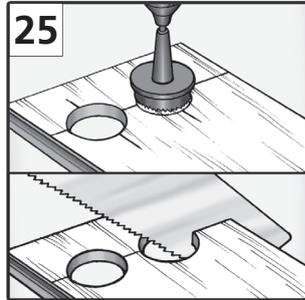
For heating-radiator pipes, holes that are drilled 3 cm / 1.2" larger than the pipe diameter must be avoided. A "fitting piece" should be cut out, glued, fitted in and fixed in place with a wedge until the glue has dried. Then cover the recesses with a radiator-sleeve [24, 25, 26].
